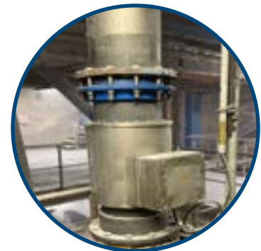
Coil with Measurement Board (Stainless Steel Housing)
